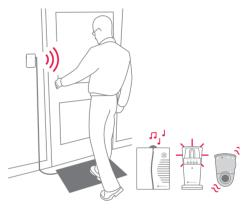
**3.** Step on the contact mat to test the installation. When the contact mat is pressed, it activates the transmitter that signals your Visit receiver. The receiver alerts you with sound, flashes or vibrations (depending on the receiver).
